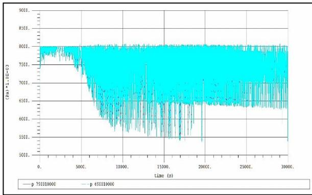
Fig. 7: Pressure Fluctuation of Secondary Circuit after SBO Condition and the SG Relief Safety Valves Opening.
