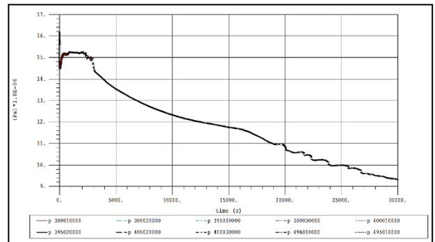
Fig. 5: Reactor Primary Pressure during Station Blackout Accident.
