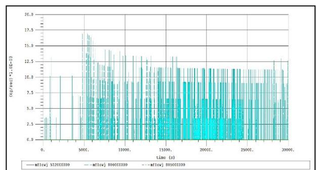
Fig. 6: The SG Relief Safety Valves A Leakage Rate During SBO Event.
