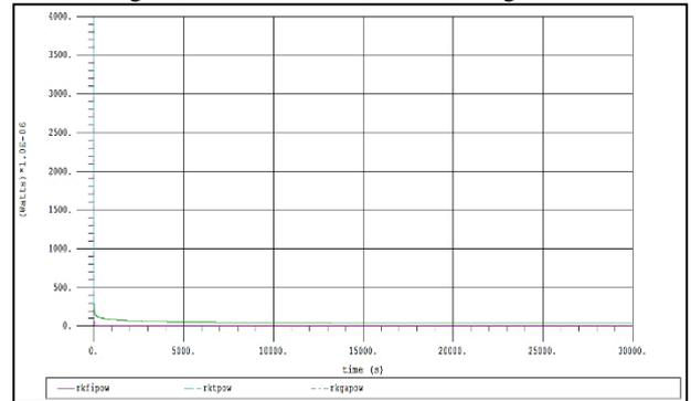
Fig. 4: Total Reactor Power, Reactor Fission Power, and Total Reactor Power from Decay of Fission Fragments and Actinides during SBO.
