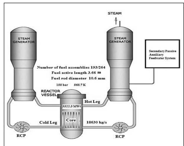
Fig. 1: Simplified Schematic Diagram of the PWR Plant and Its Main Technical Data.
