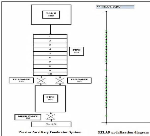
Fig. 2: Simplified Diagram and RELAP Nodalization Diagram of the Additional Passive Auxiliary Feedwater System.
