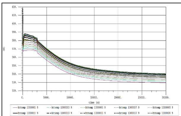
Fig. 9: Time Progression of the Cladding Temperature at Different Axial Levels.
