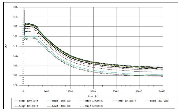
Fig. 10: The Core Temperature along Fuel Assembly after SBO Condition and the ASPAFS Operation.
