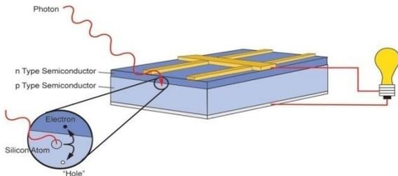
Fig. 2: Principle of photo-voltaic effect
