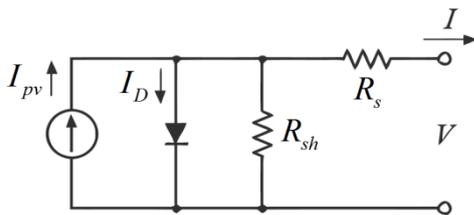
Fig. 3: PV Cell electrical representation in literature
