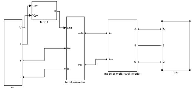
Fig. 7: MATLAB model of the proposed two stage conversion system
