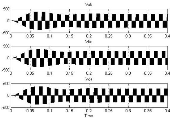
Fig. 10: Output voltage from MMC
