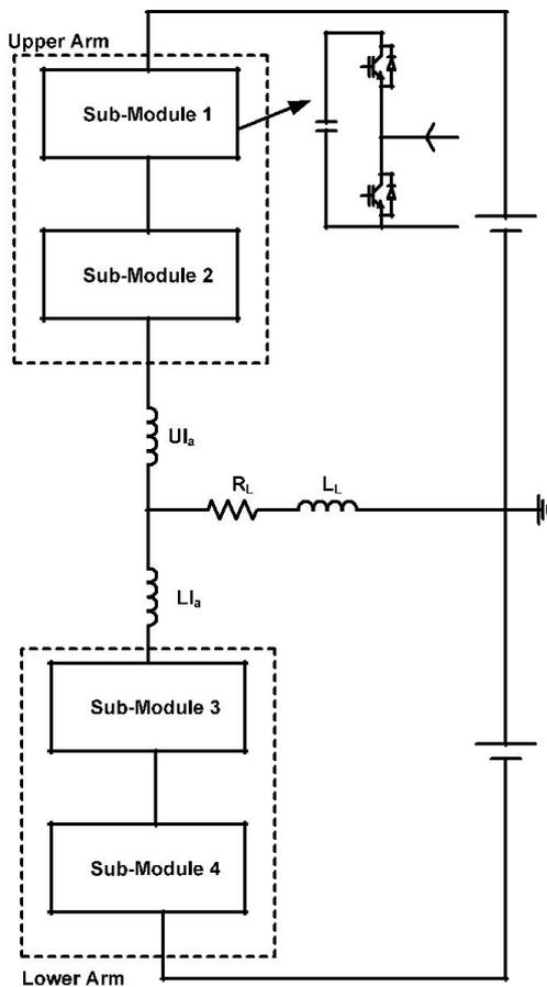
Fig. 6: Single leg of modular multilevel converter
