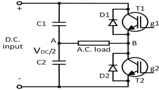
Fig. 4: Half bridge inverter
