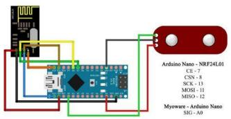
Figure 3.1 Schematic Diagram for Electromyogram Sensor
