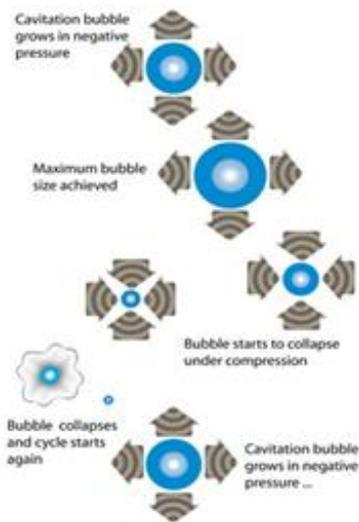
Fig. 1: The cavitation and implosion cycle [16].
