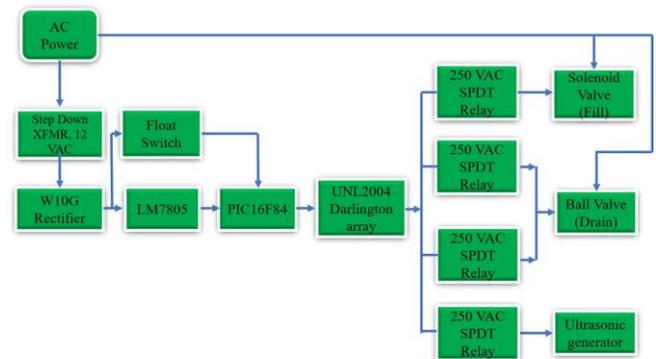
Fig. 3: The connection of the parts for the automation system.
