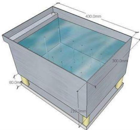
Fig. 5: The tank design and its dimensions.
