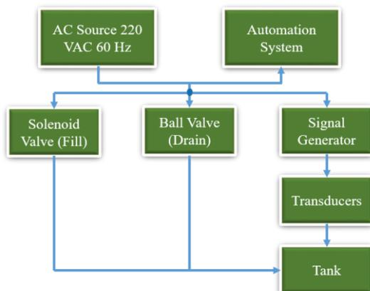
Fig. 2: The block diagram of the dishwashing system.
