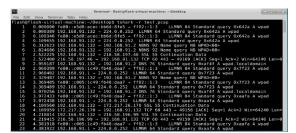
Figure 1.2: Analysing a pcap file using TShark from windows command prompt.
