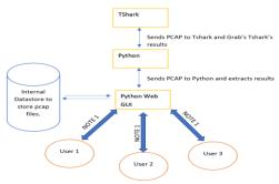
Figure 3.4: Working Procedure of this model
