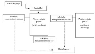
Fig. 1: Schematic Diagram for the experiment
