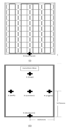
Fig. 1: Placing of thermocouples; (i) surface of panel, (ii) Back of panel
