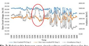
Fig. 7: Relationship between open circuit voltage and irradiance for day 1
