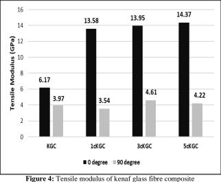
For transverse direction of fibres, the tensile modulus of KGC is 3.97 GPa, while 1cKGC is 3.54 GPa. However, further increase in the amount of nanoclay improved the transverse tensile modulus where the modulus for 3cKGC and 5cKGC is 4.61 GPa and 4.22 GPa, respectively. This shows that the addition of nanoclay in KGC does not significantly improved the transverse tensile modulus as compared to the UD tensile modulus.
