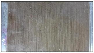
Fig. 2 : Cured Kenaf Composite plate
