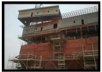
Figure 5: Picture of Modular Construction at Kencana (Erection Process) [10].
