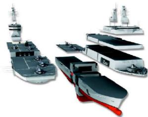
Figure 2: Modular construction concept [7]
