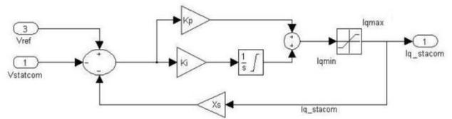
Fig 4: Voltage controller of STATCOM
