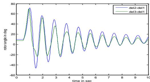
Fig (7): Relative rotor angles with Integer order FOPI controller.
