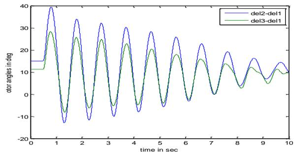
Fig (8): Relative rotor angles with Integer order PI controller.
