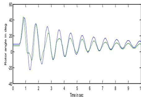
Fig (6): Relative rotor angles with Integer order PI controller
