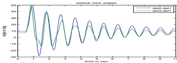
Fig(9):Relative rotor angles with FOPI controller.
