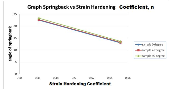
Fig. 6: Springback angle vs strain hardening coefficient, ( $n$ )
