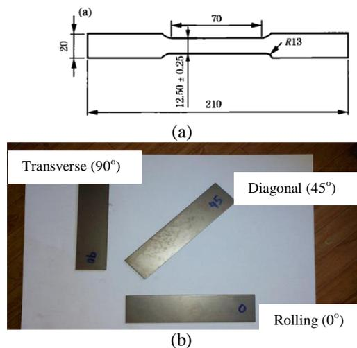
**Fig. 1:** (a) Specimen geometry for ASTM E8 tensile test, and (b) bending test
