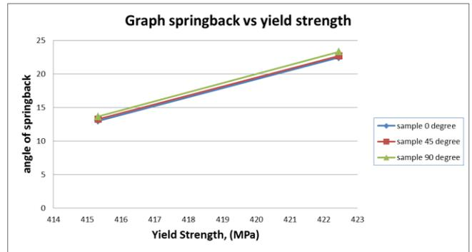
Fig. 5: Springback angle vs yield strength
