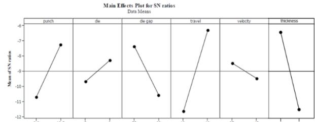
Fig. 8: Main effects plot for the influenced parameters to springback.
