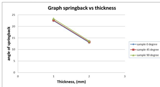
Fig. 4: Springback angle vs thickness
