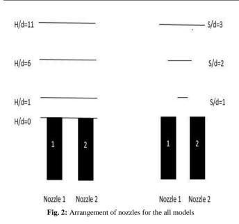
Figure 2 shows the nozzle arrangement for all nine models. The arrangement is based on the distance between the nozzles and the nozzle- plate distance (as shown in the figure). An Aluminium foil square, with surface dimension and thickness of  $300 \times 300 \times 4$  mm (as shown in Figure 3 below). The positions of thermocouples and heat flux sensor on the Aluminium flat are also shown in the figure.
