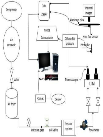
Fig. 1: Schematic of twin impingement jets tests setup
