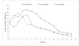
Fig. 7: Heat transfer coefficient values when S = 20 mm, and H = 10, 60, and 110 mm
