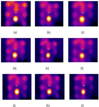
Fig. 9: Thermographic temperature distribution of Aluminium Foil Models 1, 2 and 3, (a) to (i)
