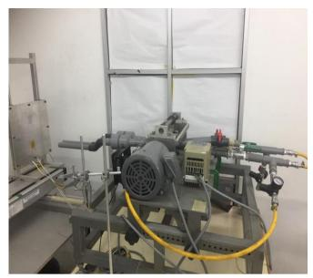
Fig. 4: Twin Impingement jets Mechanism and heat flux microsensor on the Aluminium impingement surface.
