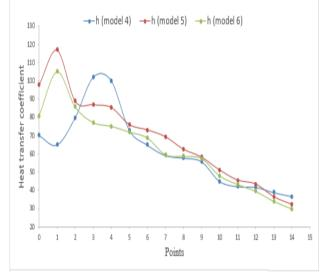
Fig. 8: Heat transfer coefficient values when S = 30 mm, H = 10, 60, and 110 mm
