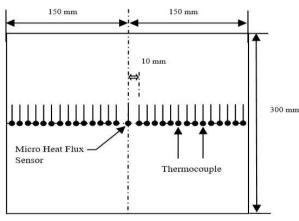
Fig. 3: Positions of sensors on the aluminium flat
