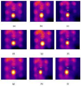
Fig. 11: Thermographic temperature distribution of Aluminium Foil Models 7, 8 and 9, (a) to (i)
