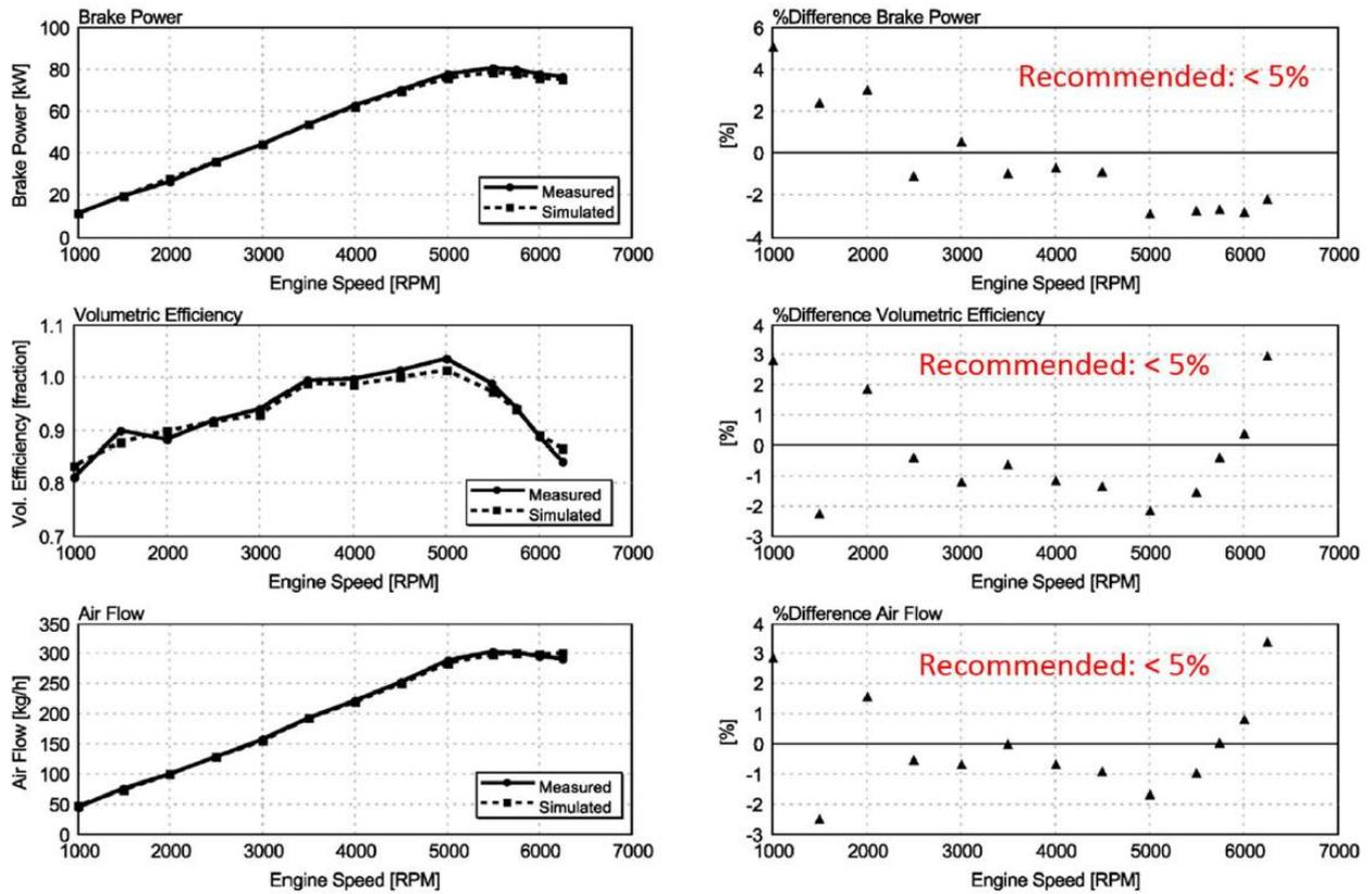
Fig. 5 Engine Performance Model Correlation
