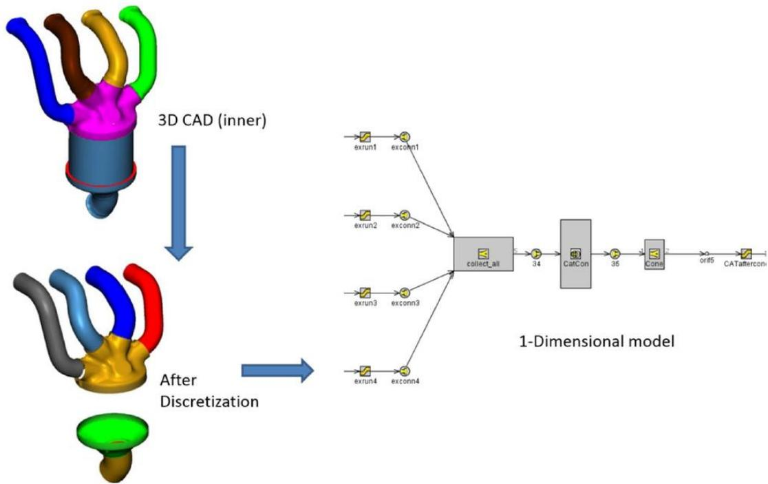
Fig. 3: Discretization of exhaust manifold
