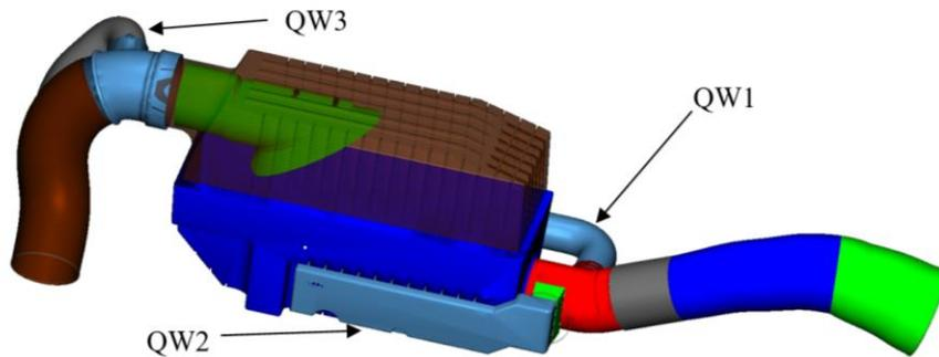
Fig. 6: Air intake module of a baseline 1600cc engine
