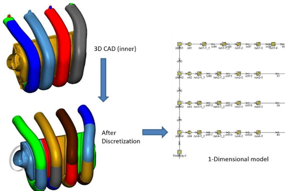
Fig 2: Discretization of intake manifold
