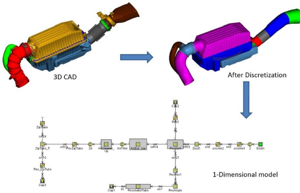
Fig 1: Discretization of air intake module
