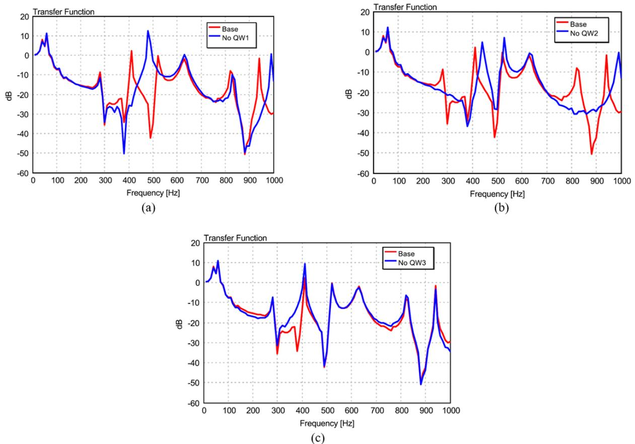
Fig. 7: Effect on transfer function when removing quarter-wavelength at a) snorkel; b) lower air box; and c) air duct
