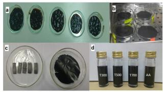
**Fig. 4:** Photograph of a) gel-like GO; b) dried GO; c) left: rGO film, right: GO film and d) rGO dissolved in DMAc, from left: thermal reduction at 300°C (T300), 500°C (T500), 700°C (T700) and ascorbic acid (AA)
