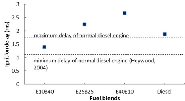
**Fig. 3:** Ignition delay of diesel-ethanol-PME blends at 1600 rpm engine speed
