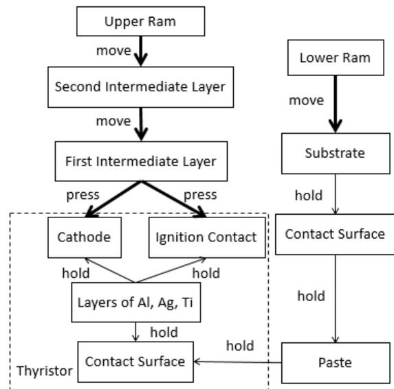
**Fig. 3:** Function analysis of pressure sintering process and components by Siemens with components of thyristor being bracketed [10].
