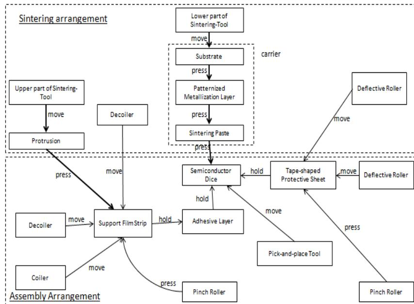
**Fig. 4:** Function analysis of Infineon patent, which includes the assembly and sintering arrangement. The substrate, paste and patternized metallization layer were bracketed as the carrier for the semiconductor module [14].
