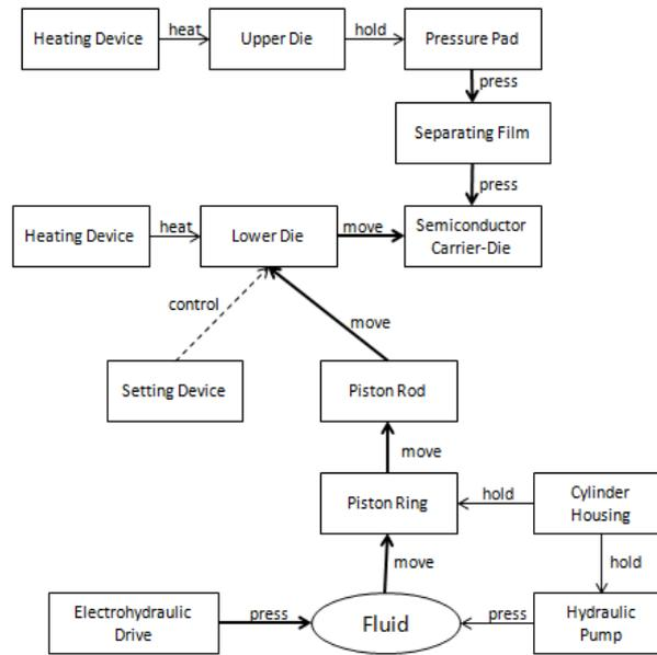
Fig. 5: Function analysis of the components in the sintering chamber of Danfoss' patent [15].
