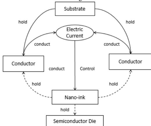
Fig. 6: Function analysis of Valtion patent [9].
