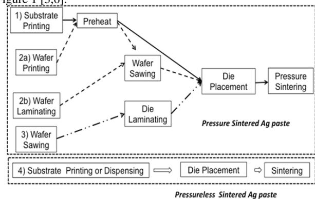
**Fig. 1:** Main processing steps for four different approaches to forming pressure assisted and pressureless sintered Ag joints [3].
