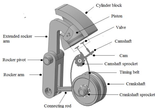
Fig. 1: A proposed design for the Crank-rocker engine geometry.
