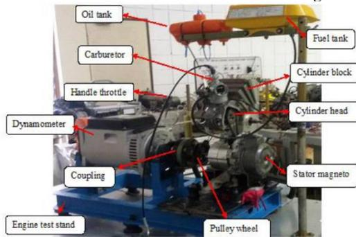
**Fig. 3:** The crank-rocker engine and the accessories on the test bed.
