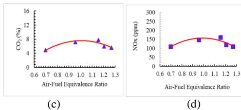
**Fig.5:** (a-d). (a) HC (b) CO (c) CO<sub>2</sub> (d) NO<sub>x</sub> emissions vs air-fuel equivalence ratio at 50% throttle and 2000 rpm
