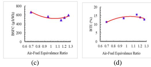
**Fig. 4:** (a-c). (a) BT (b) BP (c) BSFC (d) BTE vs air-fuel equivalence ratio at 50% throttle and 2000 rpm
