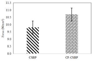
Fig. 3: Maximum force of bioplastics
