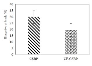
Fig. 5: Maximum elongation of bioplastics.
