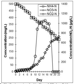
Fig. 2B: Nitrification using the bio-filter of K2 AnoxKaldnes packing material in batch reactor experiments with high concentrations of ammonium sulphate, 500 mg/L ammonia –nitrogen.
