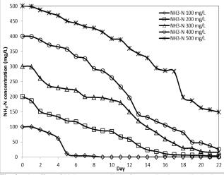
**Fig. 3:** The effect of high concentrations of ammonia-nitrogen in the batch culture with the bio-filter of K2 AnoxKaldnes packing material.
