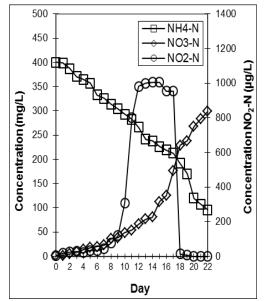
Fig. 2A: Nitrification using the bio-filter of K2 AnoxKaldnes packing material in batch reactor experiments with high concentrations of ammonium sulphate, 400 mg/L ammonia –nitrogen.
