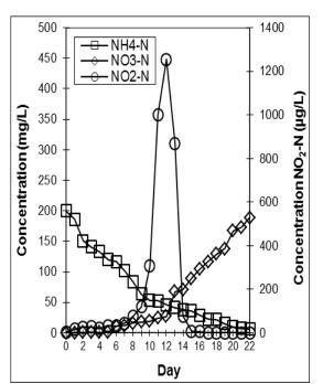
Fig. 1A: Nitrification using the bio-filter of K2 AnoxKaldnes packing material in batch reactor experiments with high concentrations of ammonium sulfate, 200 mg/L ammonia –nitrogen.
