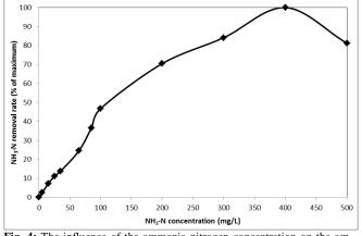
Fig. 4: The influence of the ammonia-nitrogen concentration on the ammonia-nitrogen removal rate in batch culture using the K2 AnoxKaldnes packing material.
