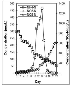
Fig. 1B: Nitrification using the bio-filter of K2 AnoxKaldnes packing material in batch reactor experiments with high concentrations of ammonium sulphate, 300 mg/L ammonia-nitrogen.
