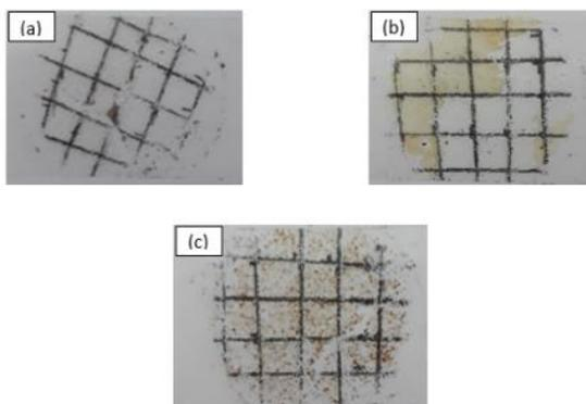
**Fig. 1:** Surface of pressure-sensitive tape after the adhesion test at sintering temperature of (a) 150°C (b) 200°C and (c) 250°C
