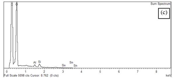
**Fig. 5:** The EDX spectrum of the elemental component at (a) 250 (b) 500 and (c) 750 ppm
