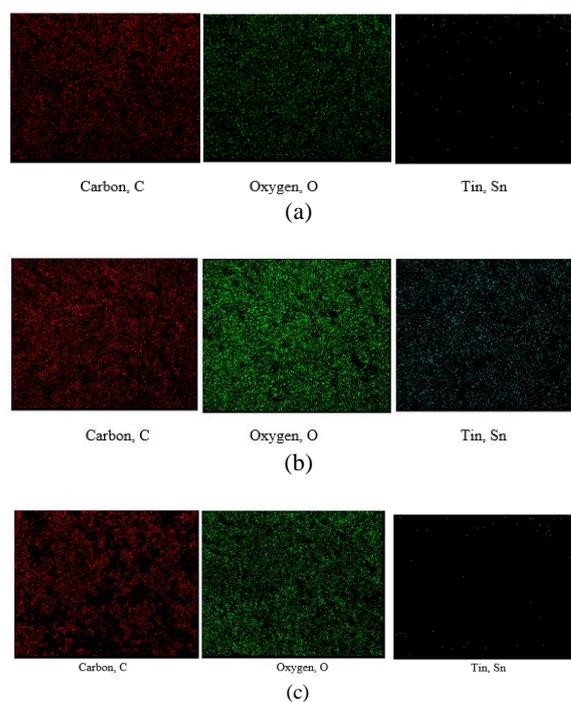
**Fig. 4:** The EDX analysis for C, O and Sn distribution on the coated layer at (a) 150 °C (b) 200 °C and (c) 250 °C
