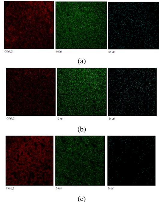
**Fig. 6:** The EDX analysis for element C, O and Sn distribution on the coated layer at (a) 250 (b) 500 and (c) 750 ppm.
