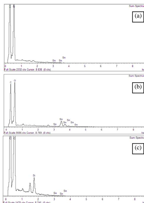
**Fig. 3:** The EDX spectrum of the elemental component at (a) 150 °C (b) 200 °C and (c) 250 °C
