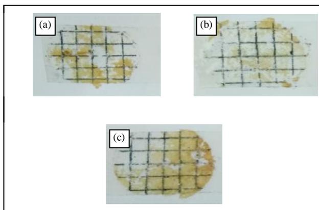
**Fig. 2:** Surface of pressure-sensitive tape after the adhesion test at tin octoate concentration of (a) 250 ppm (b) 500 ppm and (c) 750 ppm
