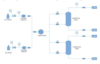
Fig. 1: Adsorption Unit Schematic Diagram
