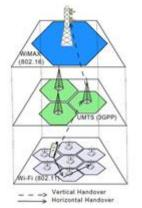
Fig. 1. Differences between Vertical and Horizontal Handover
