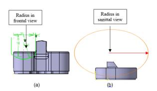
Fig. 5: (a) Radius of Tibial in frontal view (RTF) and (b) Radius of Tibial in sagittal view (RTS)
