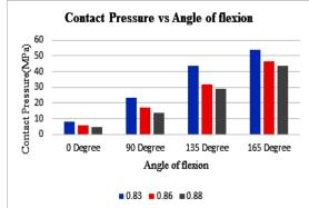
**Fig. 6:** Contact pressure (MPa) versus angle of flexion for 0.83, 0.86 and 0.88 conformity values
