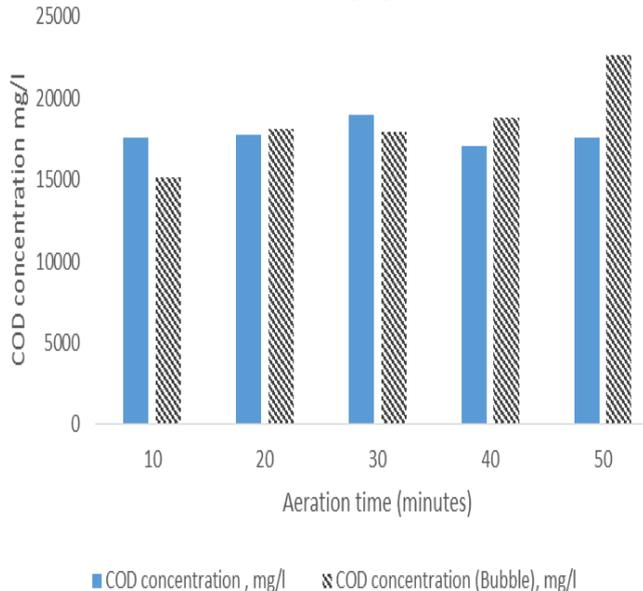
Fig. 2: Effect of aeration time on COD removal for Company A
