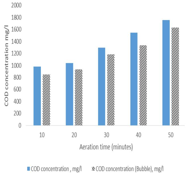
Fig. 3: Effect of aeration time on COD removal for B.
