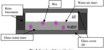
Fig. 3: Sample cell from side view
