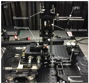
Fig 2(a): Experiment workplace
