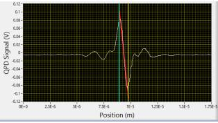
Fig. 4: Graph of QPD signal (V) versus Position (µm).
