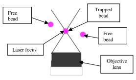
Fig. 1: Optical trapping at the focus of the laser beam
