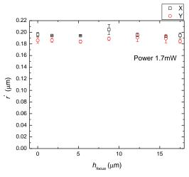
Fig. 7: Graph of effective radius ( $r^*$ ) versus focus height ( $\mu m$ ) for P=1.7 mW
