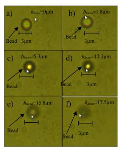
Fig. 9a-f: Sequence of trap bead at various focus height at 1.7mW laser power (white arrow indicates the laser spot).
