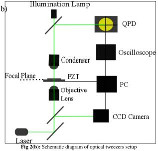
**Fig. 2:** Schematic diagram of optical tweezers setup
