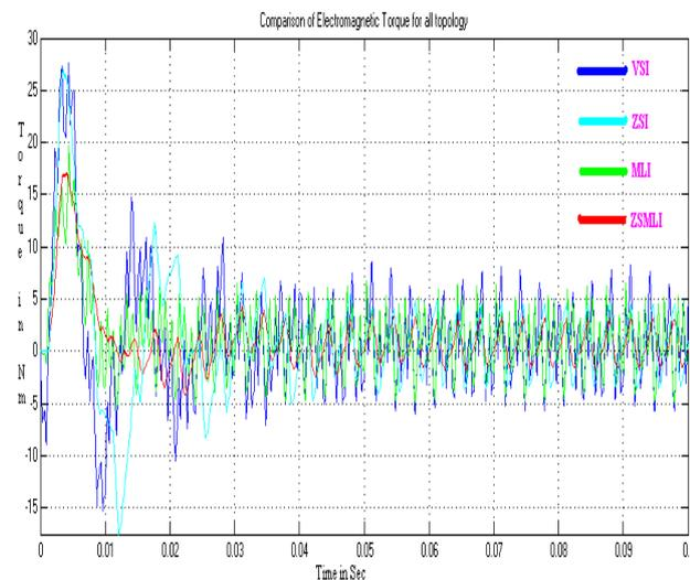
Fig. 20: Torque response curve of different topology fed BLDC motor
