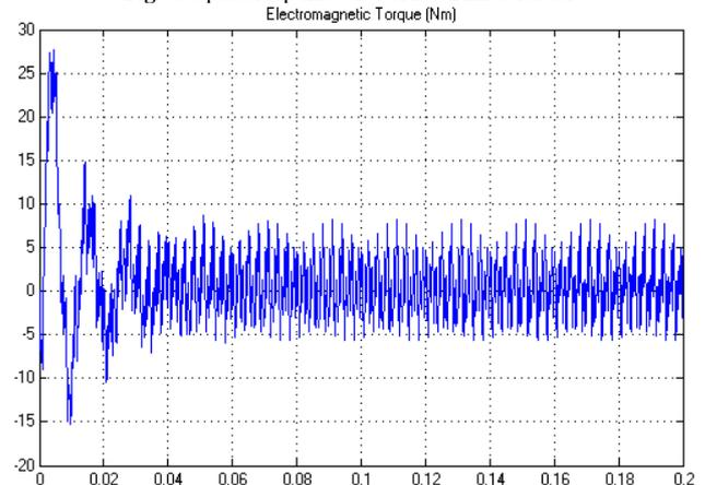
Fig. 5: Torque of VSI fed BLDC Motor
