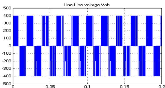
Fig. 2: Single phase output Voltage from VSI
