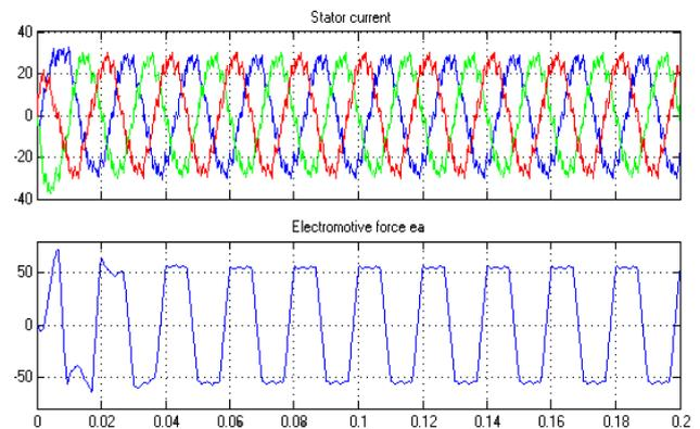
Fig. 3: Three phase stator current and Back EMF
