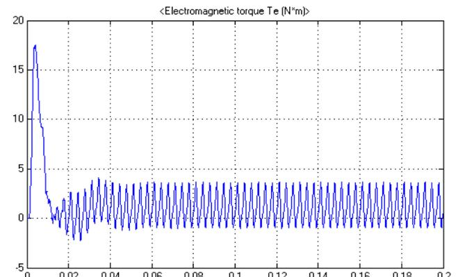
Fig. 17: Torque curve of ZSMLI fed BLDC motor
