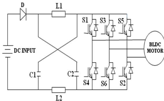
Fig. 6: ZSI fed BLDC motor
