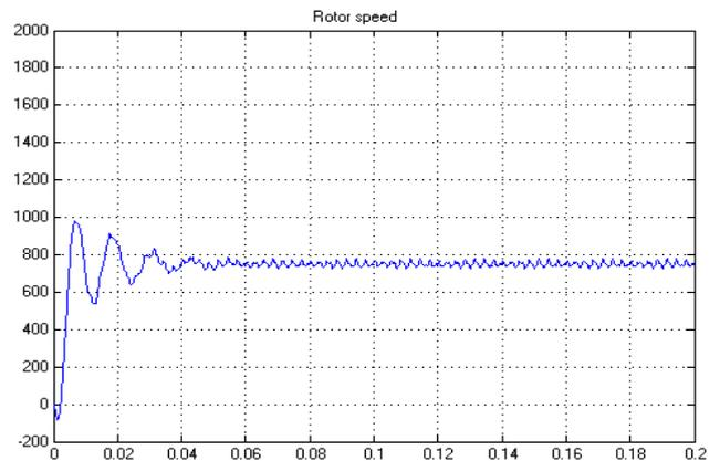
Fig. 10: Speed response of ZSI fed BLDC Motor
