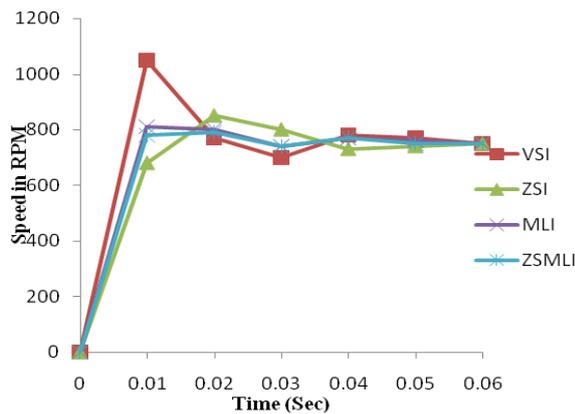
Fig. 19: Comparison of transient behavior between different topology fed BLDC motor
