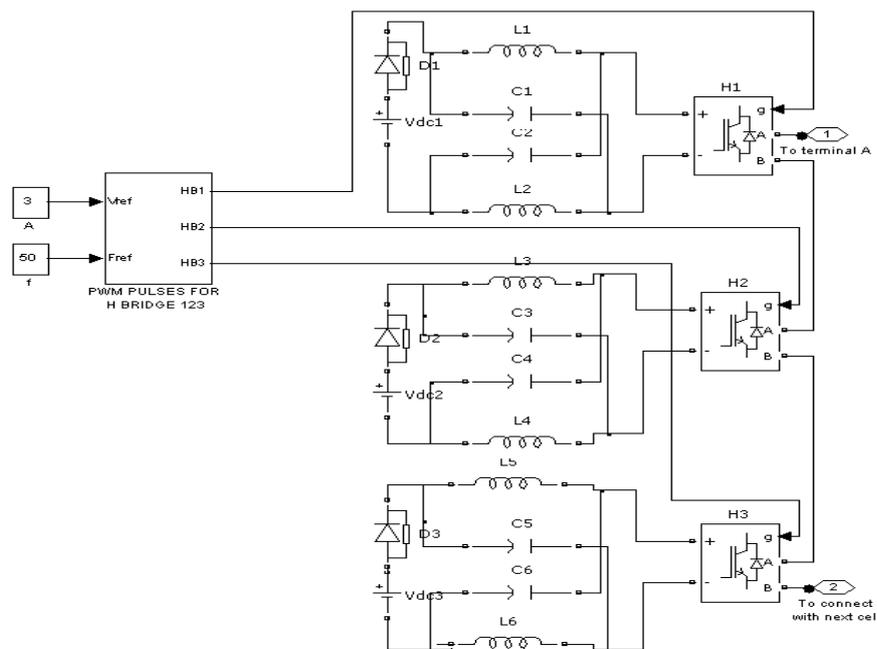
Fig. 15: Z source based MLI fed BLDC Motor
