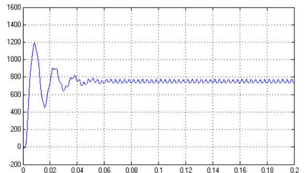
Fig. 4: Speed response of VSI fed BLDC Motor
