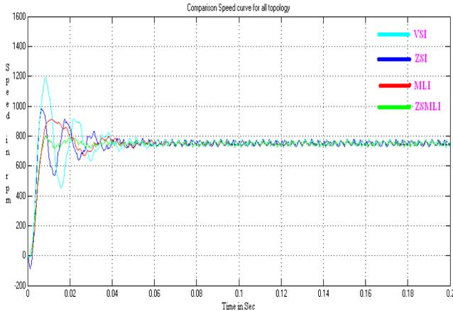
Fig. 18: Speed response curve of different topology fed BLDC motor
