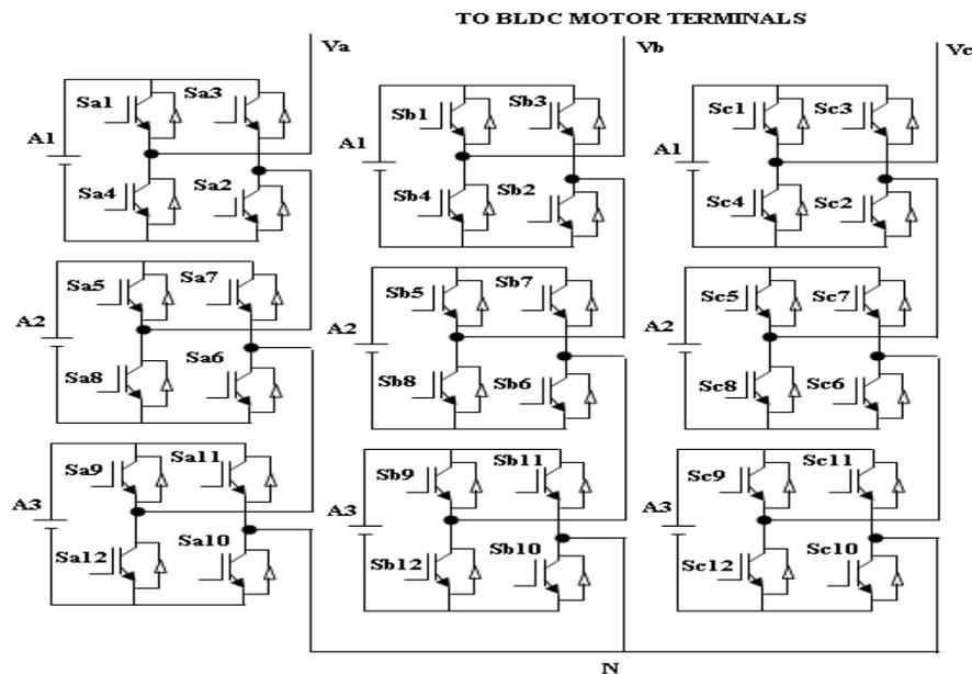
Fig. 12: Cascaded Multilevel inverter for BLDC motor
