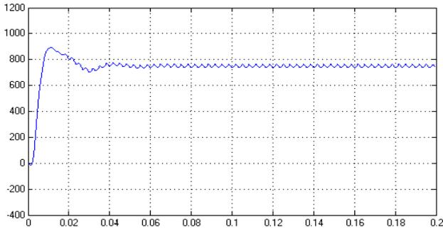
Fig. 13: Speed response curve of MLI fed BLDC motor
