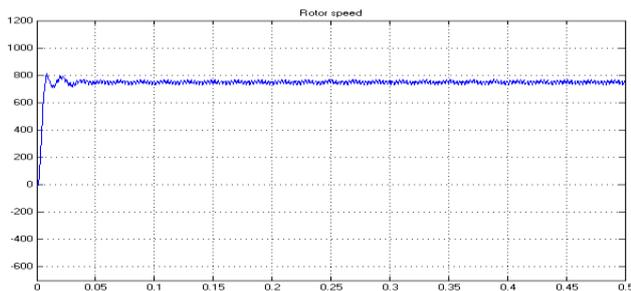
Fig. 16: Speed response curve of ZSMLI fed BLDC motor
