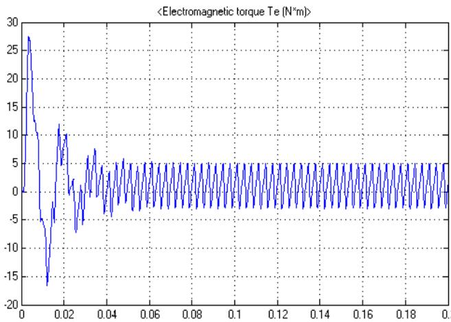
Fig. 11: Torque of ZSI fed BLDC Motor
