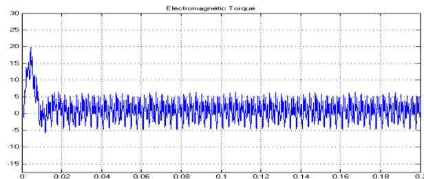
Fig. 14: Torque curve of MLI fed BLDC motor
