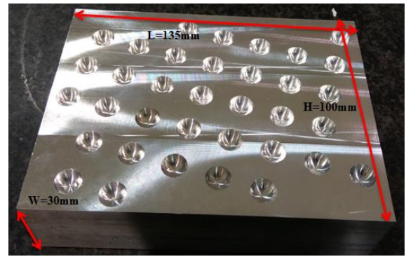
Fig. 2: Dimpled profile workpiece under study with dimension
