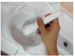
Fig 1: Crushing of the powders using pestle and mortar
