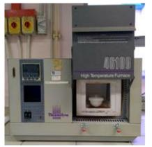
Fig 2: Calcination of as-synthesised powders
