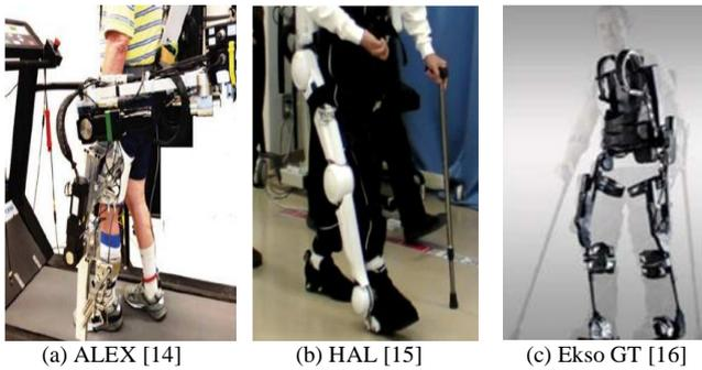
Fig. 2: A few types of single lower limbs exoskeleton
