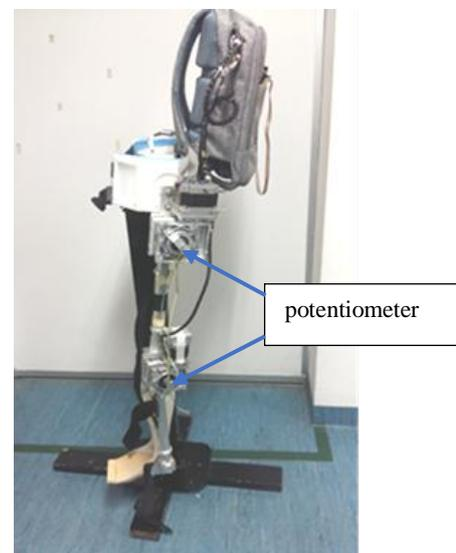
Fig. 10: Developed lower limb exoskeleton device
