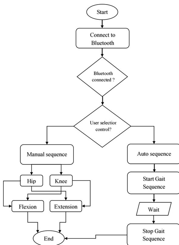
Fig. 8: Flowchart in android controlled device
