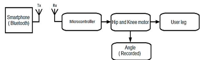
Fig. 6: Control system block diagram
