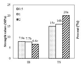
**Fig. 2:** Effects of particle size on internal bond strength (IB) and thickness swelling (TS)
