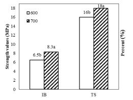
Fig. 4: Effects of board density on internal bond strength (IB) and thickness swelling (TS)
