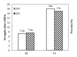
Fig. 8: Effects of hot press temperature on internal bond strength (IB) and thickness swelling (TS)
