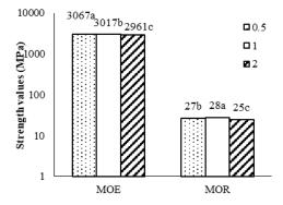
Fig. 1: Effects of particle size on modulus of elasticity (MOE) and modulus of rupture (MOR)
