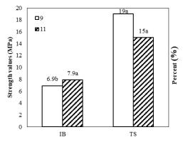
Fig. 6: Effects of resin content on internal bond strength (IB) and thickness swelling (TS)
