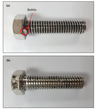
Fig 3: Surface finish of (a) 0.5 A and (b) 1.5 A.
