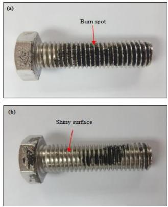
Fig 2: Surface finish when hanged (a) horizontally and (b) horizontally with rotation.
