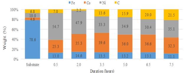
Fig. 5: Elemental percentage at different plating cycles compared with substrate.
