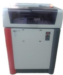
Fig. 4: Brukner S4 Pioneer machine for XRF testing
