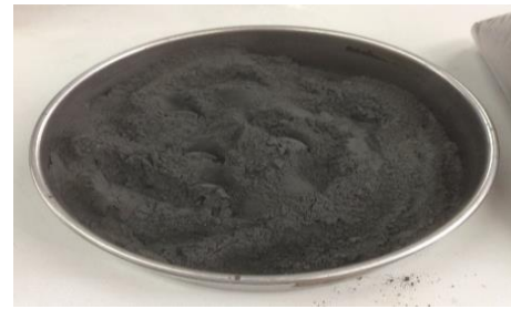
Fig. 2: Ground palm oil fuel ash (UPOFA)
