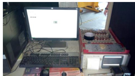
Fig. 8: Data logger system for collecting temperature data.
