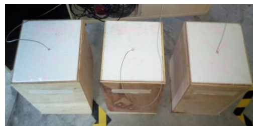
Fig. 7: Test equipment for measuring hydration temperature.
