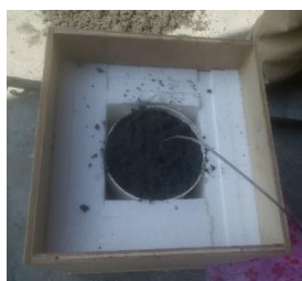
Fig. 6: Mortar is filled in an insulated cylinder.
