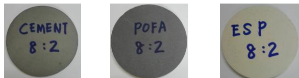
Fig. 5: Specimen pellets for X-ray fluorescent testing (a) OPC (b) POFA (c) ESP
