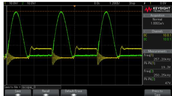
**Fig 11:** The Outcomes of ZVS for Class E Converter
