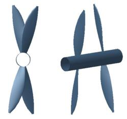
**Fig. 19:** Geomtery of the contra rotating propeller, the same propeller is just stacking without any modification in pitch blade.
