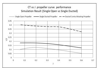
Fig. 18: Coefficient of thrust (CT) comparison of each cases
