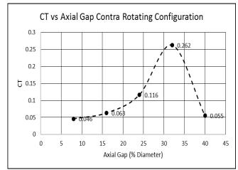
Fig. 17: Effect of an axial gap to the ducted contra rotating propeller coefficient of thrust (CT), at J = 0.4
