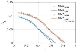
APC 10x5E and 10x7E "thin electric" propellers.
