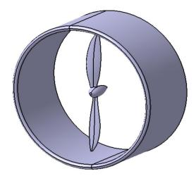
Fig. 14: Computational model of ducted propeller (duct and propeller geometry) assembly
