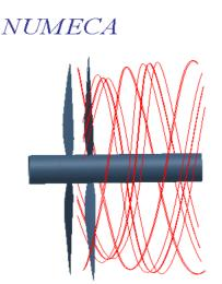
Fig. 22: Flow visualization of tip swirl flow at the ducted contra rotating (Side view)
