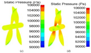
**Fig. 24:** Pressure contour taken from rear view of contra rotating configuration, Figure (a) shows Case #3.1, (b) Case# 3.2, (c) Case #3.3 (d) Case #3.4.
