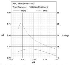
Fig. 3: Single propeller geometry: APC thin electric 10x7
