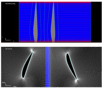
Fig. 7: Structured mesh (2D) of the contra rotating domain
