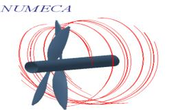
Fig. 21: Flow visualization of tip swirl flow at the ducted contra rotating (isometric view)
