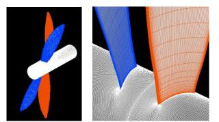
Fig. 8: the three dimensioanl of structured mesh contra rotating propeller
