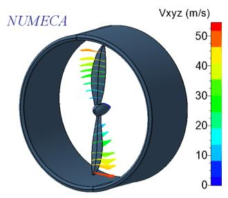
Fig. 16: Velocity distribution along the spanwise propeller
