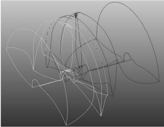
Fig. 5: Isolated propeller domain to assess the contra rotating and ducted configuration
