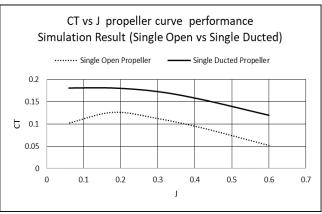
Fig. 15: Comparison CT vs J curve between single open propeller and single ducted propeller
