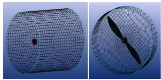
Fig. 6: Mesh that is applied on the external (stationary domain) and rotating domain of the propeller
