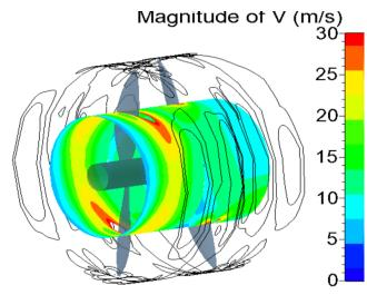
Fig. 23: Velocity contour of the contra rotating propeller domain shows the velocity change through the duct.
