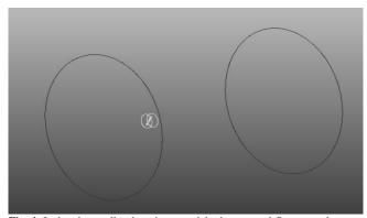
Fig. 4: Isolated propeller domain to modele the external flow over the airfoil
