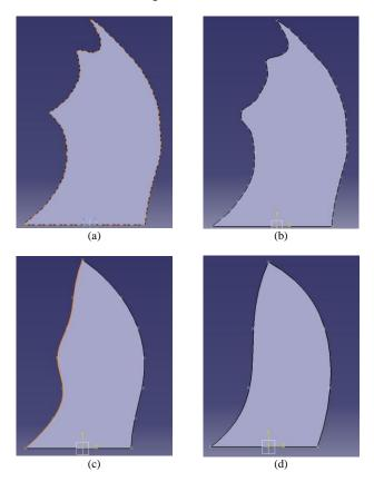
**Fig. 4**: Generated wing geometry where; (a) is the 99 vertices wing, (b) is the 49 vertices wing, (c) is the 13 vertices wing, and (d) is the 7 vertices wing
