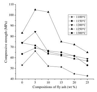
Fig. 5: Variations of the compressive strength of the samples in various compositions of fly ash and sintering temperature
