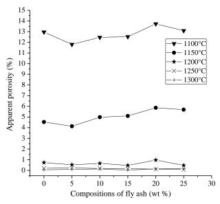
Fig. 4: Variations of the apparent porosity in various compositions of fly ash and sintering temperature
