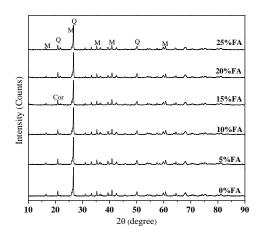
**Fig. 6:** XRD patterns of fly ash porcelain sintered at 1250 °C (M = mullite, Q = quartz, Cor = cordierite)
