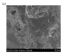
**Fig. 8:** SEM photomicrograph of fly ash porcelain bodies sintered at 1250 °C; (a) PFA5, (b) PFA15, (c) PFA25
