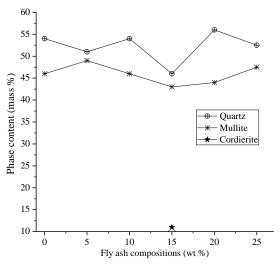
Fig. 7: Variations of phase content of fly ash porcelain bodies sintered at the sintering temperature of 1250  $^{\circ}\mathrm{C}$
