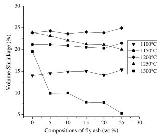
Fig. 3: Variations of the volume shrinkage in various compositions of fly ash and sintering temperature
