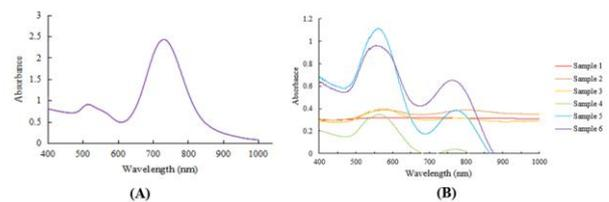
**Figure 2:** The absorbance spectra graph of the gold nanorods (A) Before centrifugation and (B) After centrifugation.
