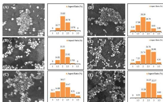
**Figure 3:** FE-SEM images of AuNRs which the centrifugation speed is varied and the bar chart shows the percentage of aspect ratio shown in the graph; (A) sample C1; (B) sample C2; (C) sample C3; (D) sample C4; (E) sample C5; (F) sample C6
