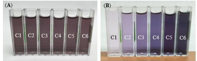
**Figure 1:** Image of the cuvette shows the result of C1 (2500 rpm), C2 (3000 rpm), C3 (3500 rpm), C4 (4000 rpm), C5 (4500 rpm) and C6 (5000 rpm) which is obtained (A) before centrifugation; (B) after centrifugation according to the assigned centrifugation speed.
