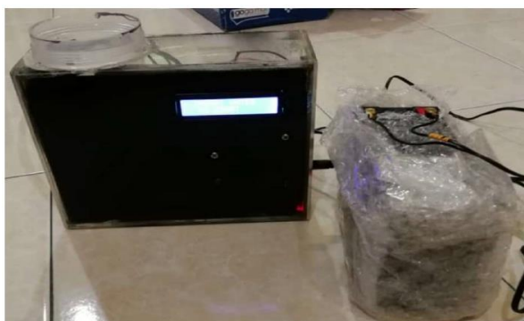
Fig. 15: The prototype of automated transfusion set for agarwood inducer.
