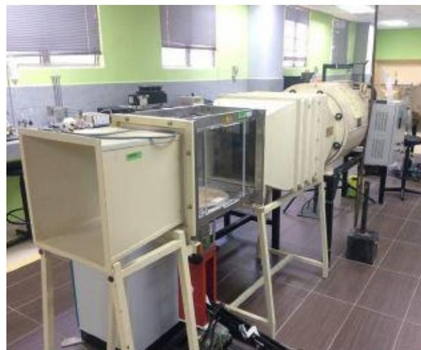
Fig. 5: The open circuit wind tunnel
