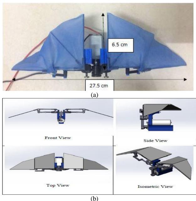
Fig. 2: (a) Fabricated MAV model, (b) CAD drawing for the MAV model
