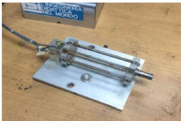
Fig. 3: Strain gauge balance unit
