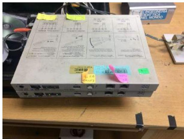
Fig. 4: Kyowa PCD-300A Data Acquisition unit
