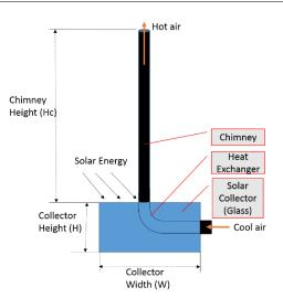
Fig. 1: Schematic layout of Green Tower.
