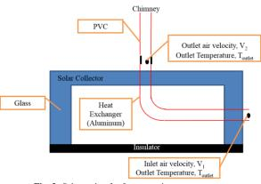
Fig. 3: Schematic of reference point measurement.
