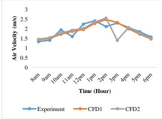
Fig. 6: Air velocity comparison between experimental, CFD1, and CFD2
