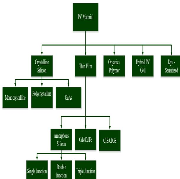
Fig.2: Classification of photovoltaic cell based on PV material [21].
