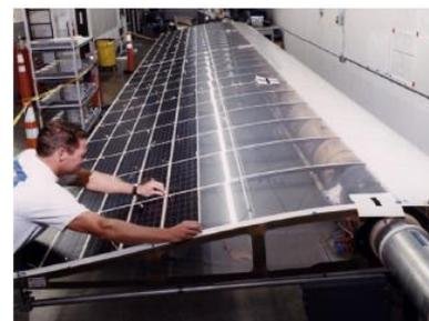
Fig. 10: Solar-powered aircraft PV installation (Helios prototype) [42].
