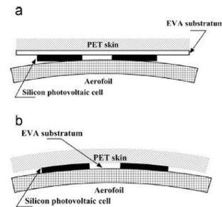
Fig. 8: Method to install on PV Cell on the airfoil shape.
