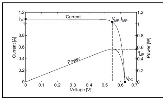
Fig.1: I-V Curve of a Solar Cell [20]
