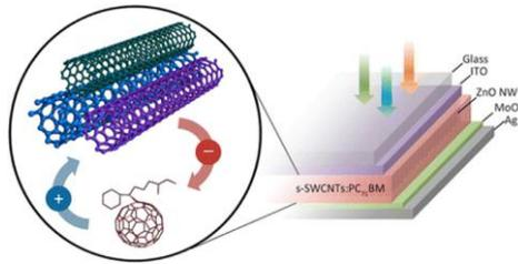
Fig. 3 Polychoral carbon nanotubes with a solar cell. [34]
