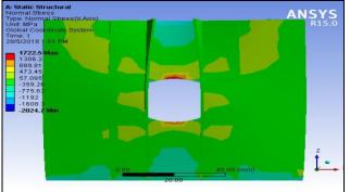
Fig. 11: Case 4: Top view of normal stress.
