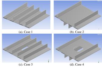
**Fig.1:** Cases of Multi-configuration stiffened panel.
