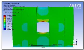
Fig. 8: Case 3: Top view of normal stress.
