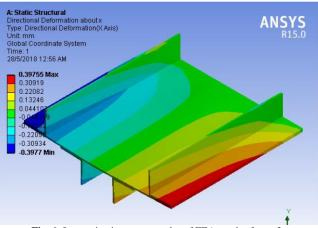
Fig. 6: Isometric view contour plot of FEA result of case 2.
