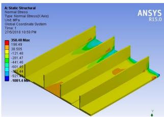
Fig. 5: Isometric view contour plot of FEA result of Case 1.
