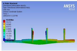
Fig. 9: Case 3: Side view of x direction deformation.
