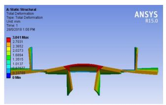
Fig. 12: Case 4: Front view of total deformation.
