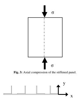
Fig. 4: Axis orientation of the stiffened panel.
