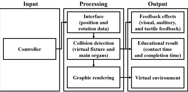
Fig. 1: Blockdiagram of EpiduroSIM™
