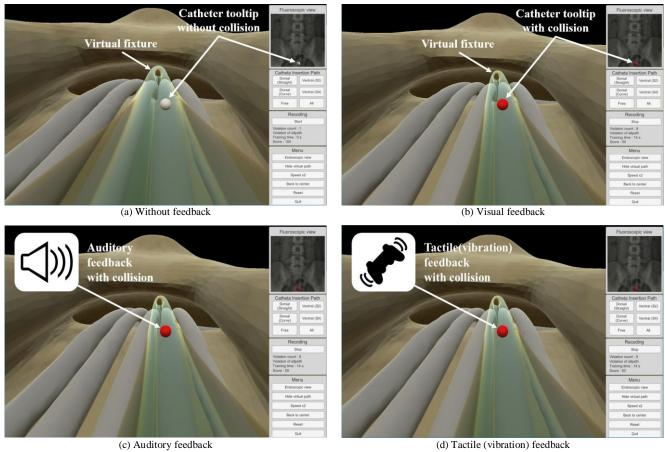
**Fig. 4:** Feedback effects applied to EpiduroSIM<sup>TM</sup>
