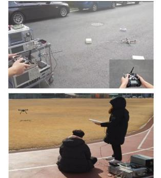
Figure 6:. Experiments for reactive jamming
