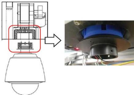
Figure 5: Lower socket detached inside the ALS
