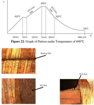
Figure 23: PCD Binding Section under 690°C (Fine)
