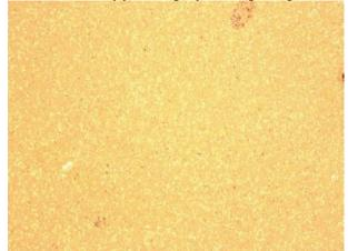
Figure 11: WEDM Process PCD Surface with Agent Preventing Electrolyte Exposure (x200)
