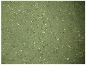
Figure 13: PCD Surface prior to Exposure to Grinding Solution
