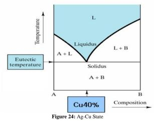
Therefore, to resolve such issue the selection of filler metal of one solid solution made of Ag-Cu-Ti is required. As a result of checking with conditional changes if the cooling time and brazing was 15[min] the most stable binding status was obtained.
