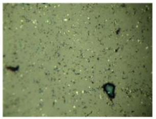
Figure 14: PCD Surface after 10 Minutes of Exposure to Grinding
