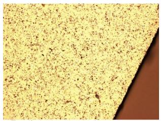
Figure 18: PCD Bite Build-up Edge after Process Improvement
