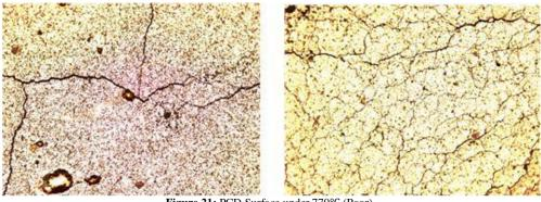
Figure 21: PCD Surface under 770°C (Poor)
