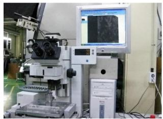
Figure 4: Toolmaker's Microscope(STM-6)
