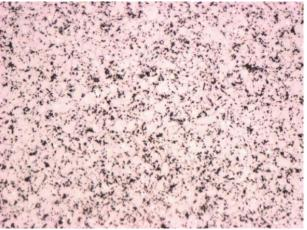
Figure 9: PCD Surface after WEDM Process (x500)
