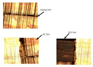
Figure 19: Case of Poor Vacuum Brazing
