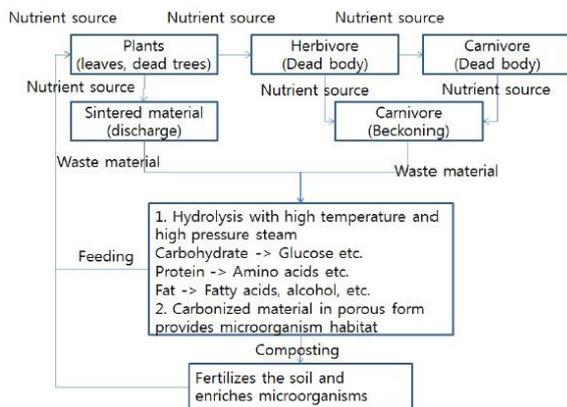
Fig.2: the concept of recycling of organic waste by high-temperature high-pressure steam
