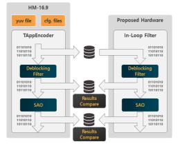
Figure 17: Verification method of proposed hardware structure
