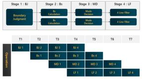
Figure 9: 4-Stage Pipeline Structure of Filtering Module
