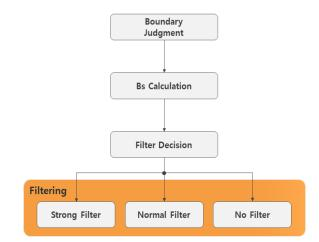
Figure 1: The process of deblocking filter
