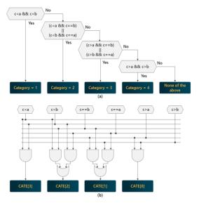
Figure 14:EO category decision method and hardware structure optimization  $% \left( {{{\left[ {{{\left[ {{{\left[ {{{\left[ {{{\left[ {{{c}}} \right]}}} \right]}} \right.}} \right]}_{\rm{const}}} \right]}_{\rm{const}}} \right)$
