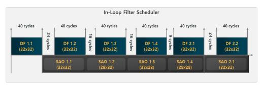
Figure 15: Scheduling of in-loop filters
