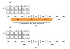
Figure 16: SAO processing sequence according to deblocking filtering order
