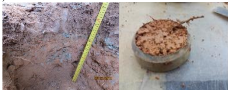
Fig. 1: Soil preparation for direct shear test
