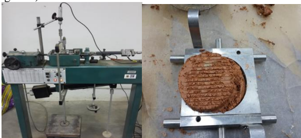
Fig. 2: Strain-controlled direct shear test machine with the shearing box
