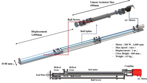
Figure 2: Telescopic Linear Actuator
