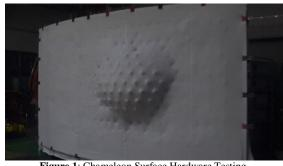
As shown in [Figure 1], the chameleon is composed of a stretchable screen and a telescopic linear actuator[8] module and an entire frame, and that has a continuous surface rather than a segmented representation. The travel distance of the actuator 1 meter to the total screen size can represent a three-dimensional shape than other pin-screen displays. For this reason, a highly resilient screen material study was carried out at the same time, named Surface Skin.
