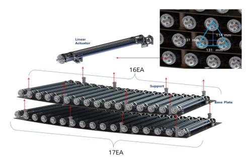
Figure 3: Structure of Telescopic Linear Actuator
