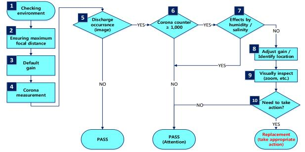
Figure 7: Ultraviolet corona determination criteria (plan)
